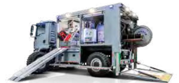
SPECIAL VEHICLE (4x4) FOR TRANSPORTING EXPLOSIVES, EQUIPPED WITH AN EXPLOSION-RESISTANT GAS-TIGHT CONTAINER
